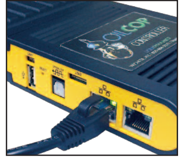
Image 1 – Controller "A" LAN Port
