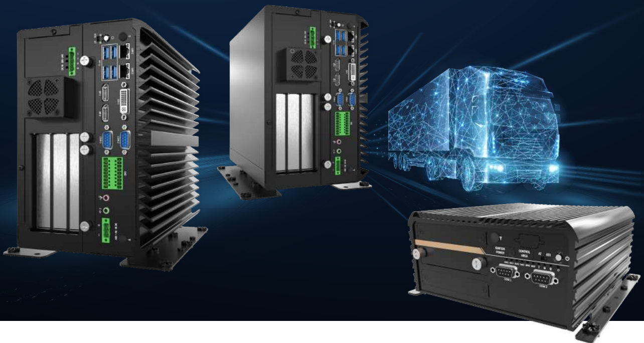
Figure 1. The Premio rugged fanless telematics computer featuring an Intel Broadwell-U processor. Source: Premio
