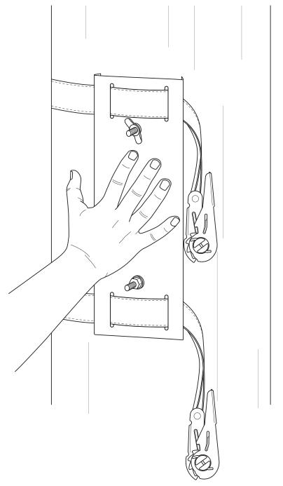
Hold column mounting bracket to the column where you would like to mount the TV.
