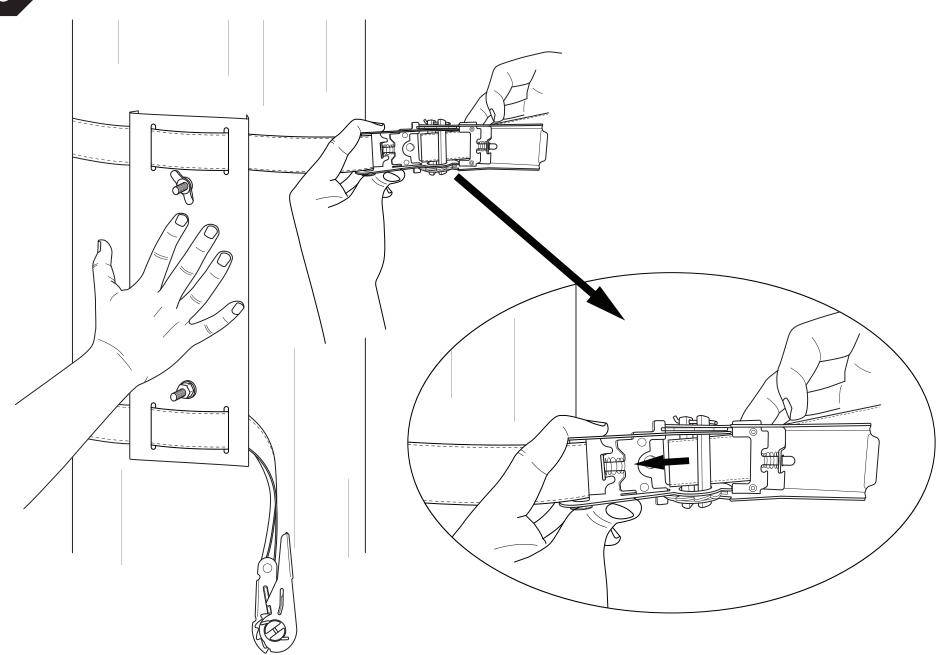
Person #2 should insert free end of strap into the slot of the ratchet buckle.
