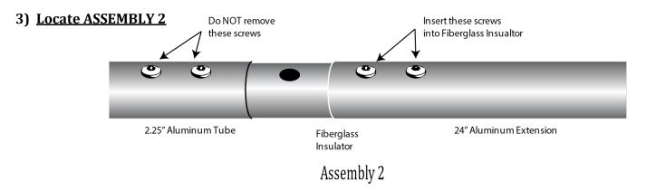
a) Slide extension away from Aluminum Tube to expose Fiberglass Insulator. Align holes in Extension with holes in Fiberglass insulator and insert 4 screws (included in packaging)
