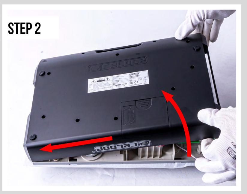
Lift the bottom cover from the right, as shown on the picture above.
