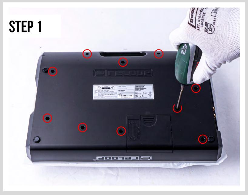
Remove all screws from the bottom housing.
