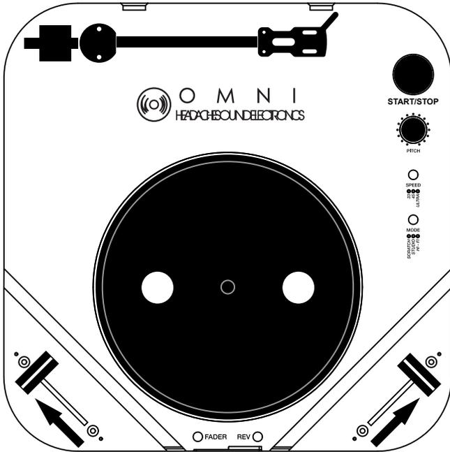
**2** PRESS AND HOLD (FADER) AND (REVERSE) BUTTONS UNTIL YOU HEAR A TONE FROM SPEAKER. RELEASE (FADER) AND (REVERSE).
