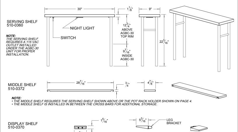
**NOTE:**THE DISPLAY SHELF IS INSTALLED ON THE SUPPORT LEGS OF THE SERVING SHELF OR THE POT RACK HOLDER SHOWN ON PAGE 4.
