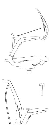
Install the back frame onto the seat frame using the 2 pins. Gently tap the pins using a mallet to securely seat the pins.
