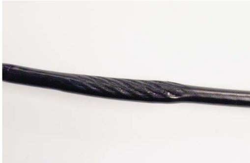
"NECKING", STRETCHED CABLE COVERING
