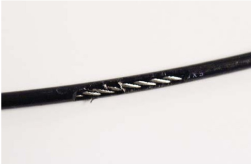
A TEAR IN THE CABLE COVER
