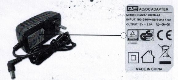
12V adapter used for 2.3inch timers or bigger ones. 6V adapter used for 1.8inch timers or smaller ones. 5V adapter used for 1.5inch timers or smaller ones.
