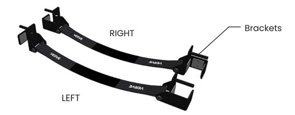
Each strap should have one bracket positioned on the outside of the uprights, and one positioned on the inside of the uprights. This will prevent the straps from swinging if a barbell is dropped on them.
