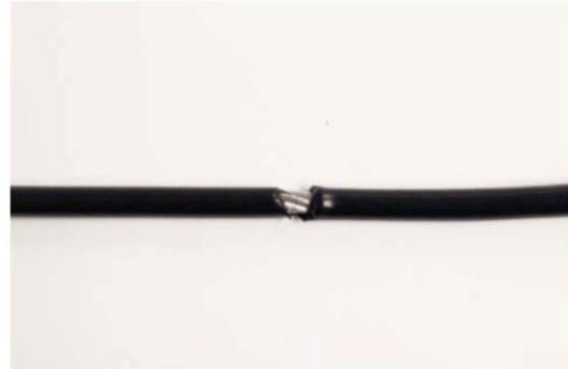
A CRACK IN THE CABLE COVER
