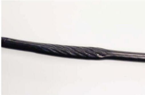
"NECKING", STRETCHED CABLE COVERING
