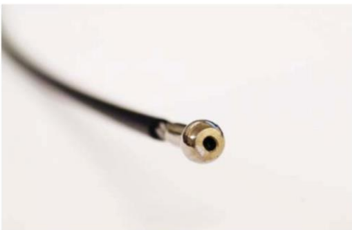
CABLE END SLIPPING OUT
