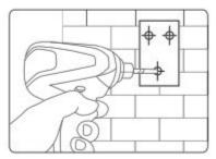
1. Place the mounting sticker in a location where the product will be installed to. Then drill 3 holes into the guides shown on the mounting sticker.
