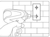
Place the mounting sticker in a location where the product will be installed to.
