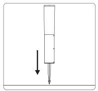
4. Position the ground spike and press firmly to secure the solar garden light into the ground.
