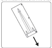
Pull the ground spike out from inside the lower section.
