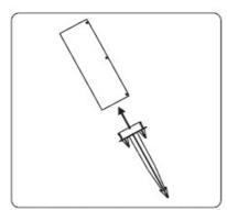
2. Carefully insert the ground spike into the lower section matching the notches together.
