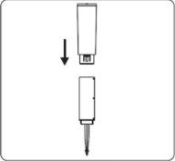
3. Carefully insert the lighting section into the lower section matching the notches together.
