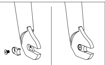
Step 2: Carefully thread in the screw with a 3mm Allen key until tight and the adapter sits flush to the dropout
