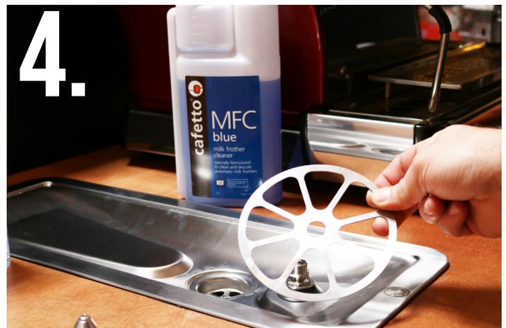
4. Remove the Actuator Plate.
