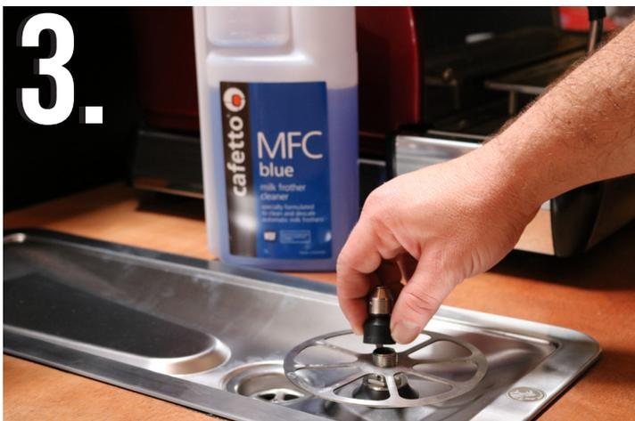
3. Unscrew the spray valve from the rinser body.
