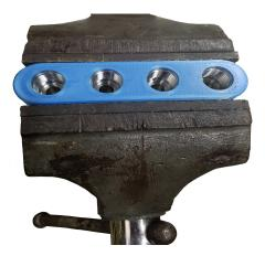
Step 4: Apply thread sealant or teflon tape to the threads of each nozzle then thread them into the coupler assembly. Do not over tighten the vise or allow the QC plugs to rotate while tightening or damage to the coupler could occur.
