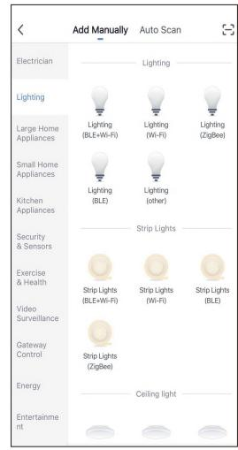
3. If the LED is not flashing when turned on, long press and hold the Reset button for more than 5 seconds. The LED will then flashes. While the LED is flashing go to the APP 'adding lighting' interface and match the LED.
