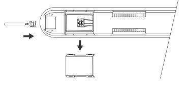
5. Remove the cover on the other end to select the light output, 3 CCT (3000K/4000K/6500K) options are available.
