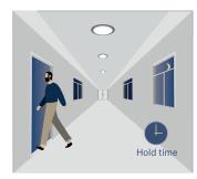
The sensor turns the light off automatically after the hold time when there's no motion detected.
