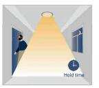
When there's no motion detected, the sensor keeps the light on at 100% for the duration of the hold time.
