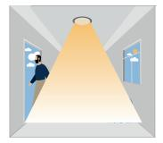
The sensor keeps the light on for the hold time after moving object leaves the detection area.
