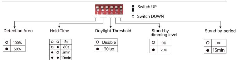
**Detection area** – The area in which movement is detected, triggering the sensor. 100% detection is also known as the maximum distance or area covered by the sensor.
