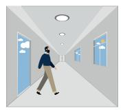
With sufficient daylight, even when motion is detected, the light remains off.
