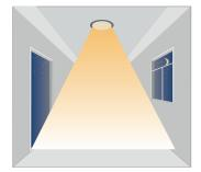
With insufficient daylight, the sensor turns the light on when motion is detected
