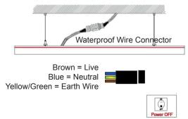
4. Wire the light unit to a mains voltage supply and adjust the light to the desired position. Turn on the power to the unit to ensure the light is working properly.
