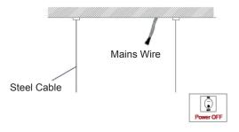
2. Screw the steel cable onto the ceiling.
