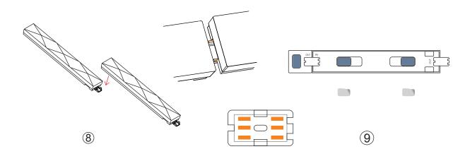
6: Finally, tear off the double-sided tape of the controller, buckle the connector, and install the controller on the connector of the first head. Installation is complete. Figure (9) Plug the adapter into the DC socket of the controller and start the experience. Figure
