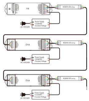
Note: If the power repeater is over heat or short circuit, the LED indicator will blink.
