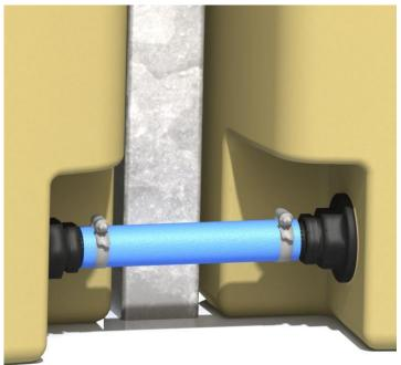
rubber tank seals at the top to enable overflow from tank to tank, however, with the proximity of the tanks this is quite hard to install.
