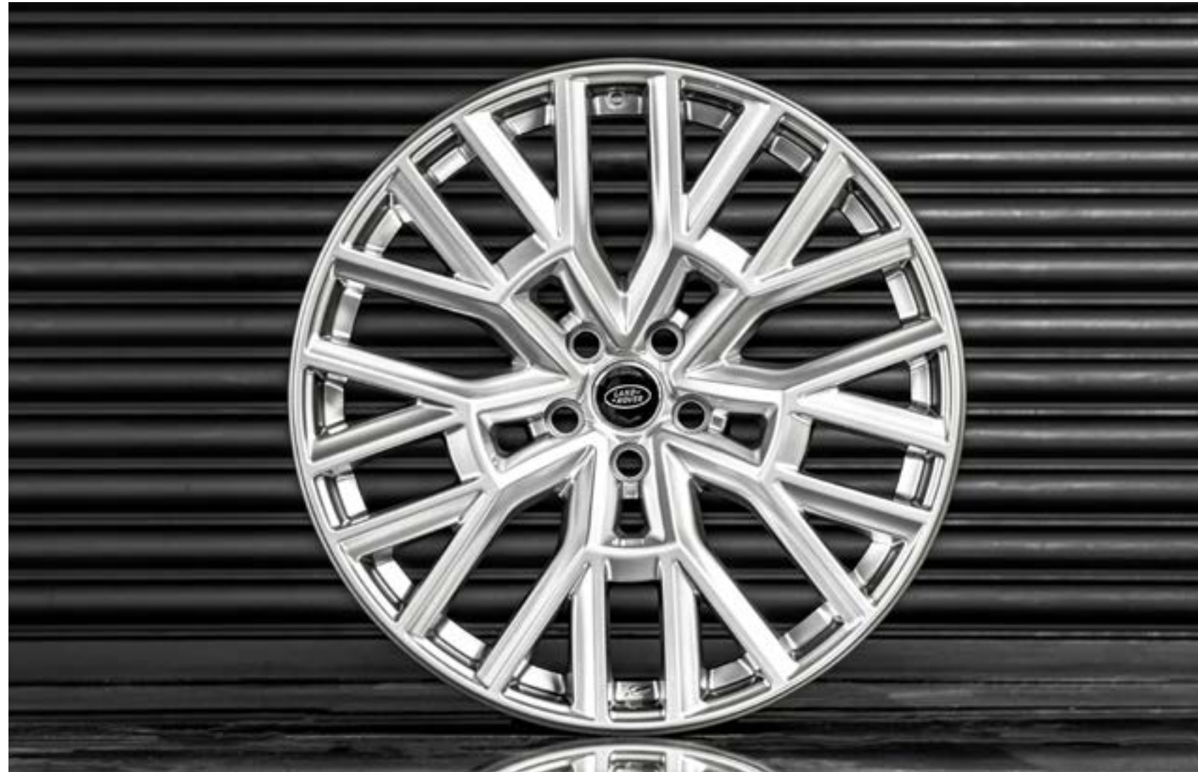
RS 3.0 SIZE FRONT WHEEL: 9.5 X 22" SIZE REAR WHEEL: 9.5 X 22" COLOUR: SHADOW CHROME PART NUMBER: WAK2F9257S1C
