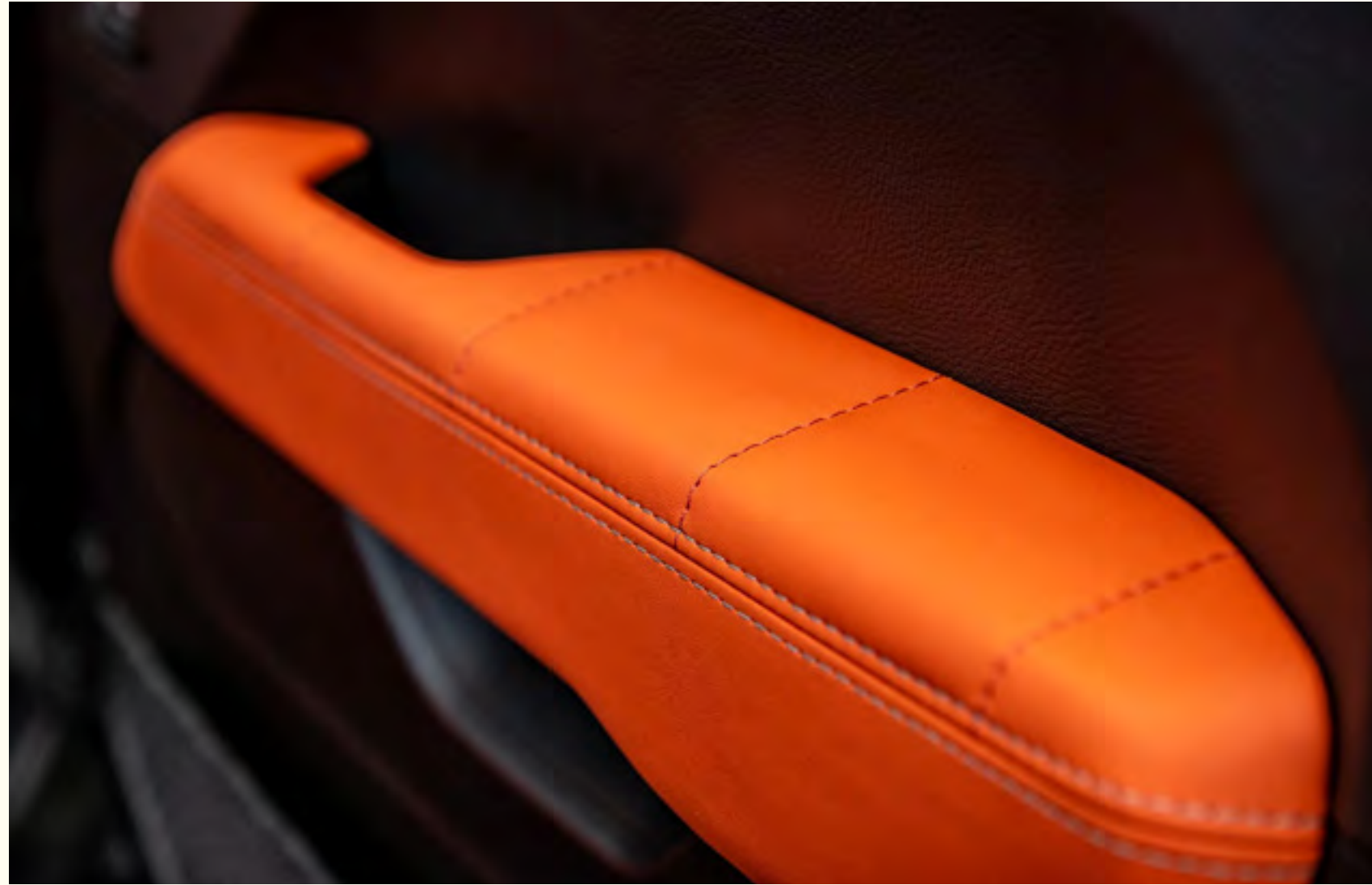
DOOR ARMRESTS COLOUR: VOLCANIC BURNT ORANGE DOOR ARMRESTS: REUPHOLSTERED IN LEATHER PART NUMBER: L129679
