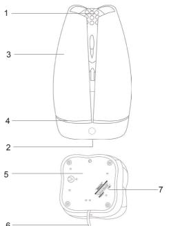
It is possible to adjust the light intensity/color using the night light intensity touch sensor (2) located at the position indicated by the illustration above. The light does not intervene or has any relation with Airfree's  $TSS^{TM}$  patented sterilization core functioning.
