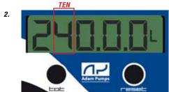
3. Insert "units" delivered: enter the number of units actually delivered, press the Total button to increase by one unit, and press the Reset button decrease by one unit, do not give any input for 5 seconds to move to the next step.
