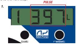
2. Insert "tens" delivered: enter the number of tens actually delivered, press the Total button to increase by one ten, and press the Reset button to decrease by one ten, do not give any input for 5 seconds to proceed to the next step.
