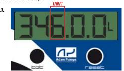
4. Insert "tenths" delivered: enter the number of tenths actually delivered, press the Total button to increase by one tenth, and press the Reset button decrease by one tenth, do not give any input for 5 seconds to move to the next step.
