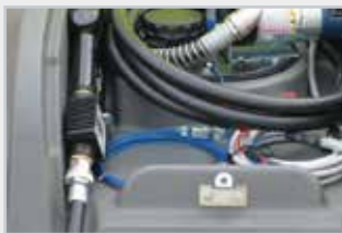
Anti Static Earth Strap - Prevents static build-up and potential of ignition while refuelling
