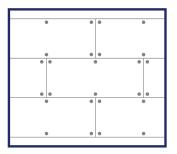
On metal decks the long edges should be laid at right angles to the corrugations. All board joints should be fully supported by the deck.
