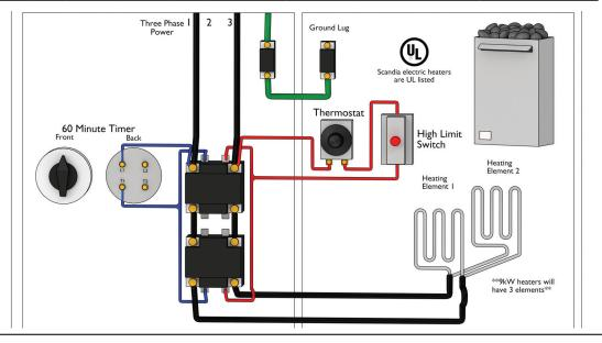
For supply connections and control panel to heater connections, use wires suitable for at least  $194^{\circ}$  F ( $90^{\circ}$  C)
