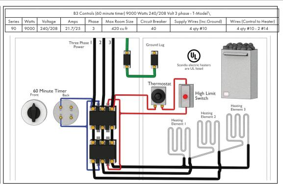
For supply connections and control panel to heater connections, use wires suitable for at least 194° F (90° C)
