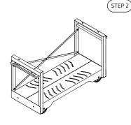
The second step is to join the sides by means of the cross bars support. When screwing, leave them almost unadjusted, you should adjust them once the grill is located.
