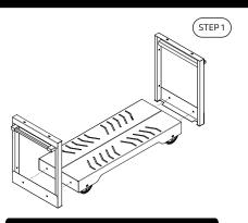
The first step in assembling the structure is to join and screw the sides to the base.
