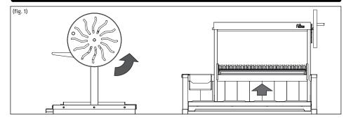
To lower the frame, the safety catch must be unlocked, holding it up and turning the steering wheel in the opposite direction to the elevation, as shown in figure 2.
