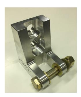
Once everything is welded in and you are ready to mount the shocks be sure not to forget that there are two flat washers that go on either side of the lower shock bearing, these will keep the shock bearing from gouging into the aluminum shock mount once they are tightened up. Before going for a road test double check your clearances and that all of the fasteners are tight. Enjoy!
