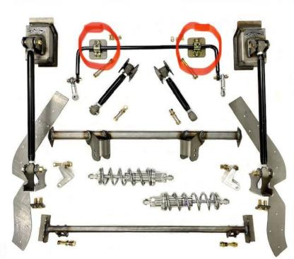
Sway bar mounting is made easy by installing your two square plates with supplied 5/16" bolts to the original upper shock mointing location. Your sway bar frame mounting will bolt to these plates using the same bolts. Circled above in the photo.
