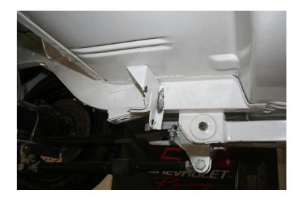
Once the e-brake cable bracket has been removed you can now install the torque boxes. You will notice in the above photo that there is a raised emboss in the floor. You will need to either flatten that surface or make a cut out in the torque box to allow it to fit snug against the floor. Note that the open end of the T-box will face the frame rail.
