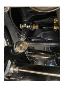
Your end links will mount using the supplied 4" long 1/2" bolt. This same bolt is the upper arm mounting bolt for the rear end. In the first photo you will see the small aluminum spacer applied next. Now your 1/2" rod end will follow with another aluminum spacer, flat washer and finally the lock nut.
