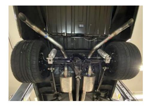
With the use of the DSE mini tubs our 4-link has plenty of clearance to allow a 315 Tire on 66/67 and a 295 tire on the 62-65 Nova.
