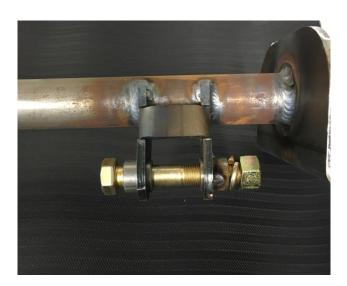
When mounting the upper shock you will need to install the ½" bolt, washer and adjustable spacer as shown in the above photo.
