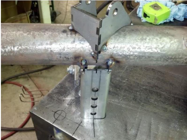
When tacking into place the lower mounting bracket it is a good decision to install the lower arm end link bushing and snug with the supplied bolts. This will ensure that the bracket will be welded at the proper width.
