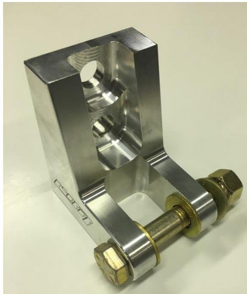
Once everything is welded in and you are ready to mount the shocks be sure not to forget that there are two flat washers that go on either side of the lower shock bearing, these will keep the shock bearing from gouging into the aluminum shock mount once they are tightened up. Before going for a road test double check your clearances and that all of the fasteners are tight. Enjoy!
