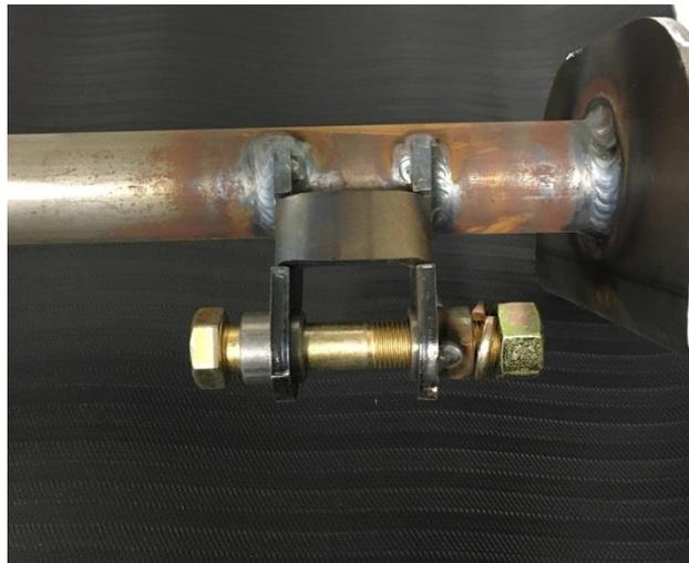
When mounting the upper shock you will need to install the 1/2" bolt, washer and adjustable spacer as shown in the above photo.
