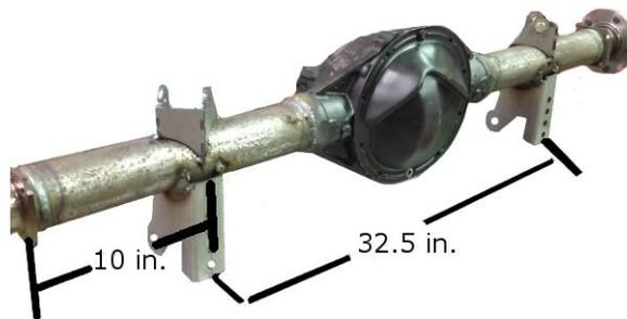
The upper mount will also use the same 10" center mark. Using an angle finder be sure to set the lower and upper brackets on the same plane or angle as the differential. Locate and ensure the angles are correct and tack weld, double check and then weld the brackets completely taking your time so as not to warp your axel tube.
