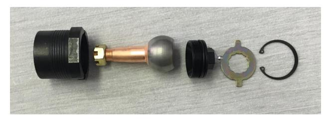
Pictured here is your lower ball joint assembly. Housing, ball stud, threaded cap, lock plate and c-clip. If replacement or adjustment is ever needed the process to adjusting out the lash or play in the stud is as follows:
