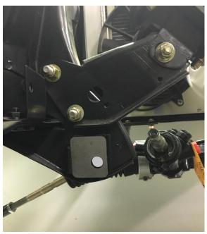
Your final adjustments will be made with the link adjuster, loosen the jam nuts, lengthen or shorten the arm as needed to get the desired setting and re-tighten the jam nuts.
