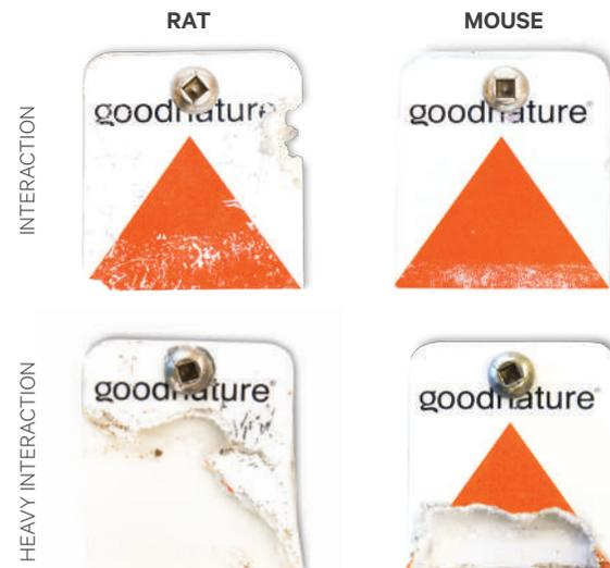
**RATS** and **MICE** are meticulous nibblers. They will often focus on one area, occasionally removing some plastic. A longer jaw length allows rats to mark further into the DETECTION SURFACE from the edge than mice.
