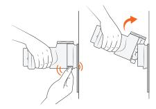
reach down through the top of the trap and push the Trigger to one side. If there is still gas in the trap, the orange Striker will be triggered, if nothing happens, all gas has been flushed out and the trap is safe to move.
