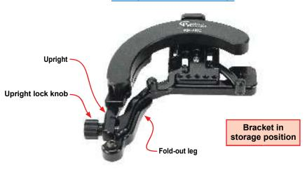
Remove your camera and flash prior to storage. It is not necessary to remove a flash cord if attached to the flash mounting plate. Loosen the upright lock knob and rotate upright backward to lower until flat. Fold in the leg.
