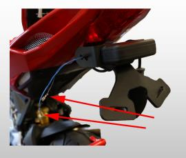
9. Assemble both indicators do not fit indicator spacer just use the rubber mount and M5 x 12 screws supplied.
