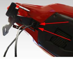
8. Thread the indicator wire through the centre hole and position the wires to the left and right. see picture
