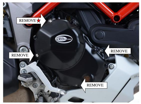
In this kit there should be: 1x Engine Case Cover (ECC0205) 2x M6 x 40mm Long Button Head Bolts 1x M6 x 90mm Long Button Head Bolt 1x M6 x 100mm Long Button Head Bolt 1x M6 Washer
