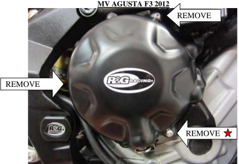
In this kit there should be: 1 x Engine Case Cover (ECC0147) 3 x M6x35mm long button head bolts 1 x M6 Washer
