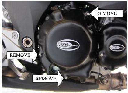
In this kit there should be: 1 x Engine Case Cover (ECC0144) 3 x M6x40mm long button head bolts 3 x M6 Washers
