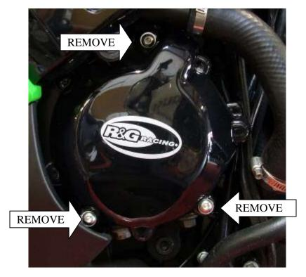
In this kit there should be 1 x Engine Case Cover (ECC0038) 3 x M6x45mm long button head bolts
