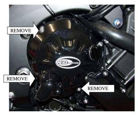
In this kit there should be 1 x Engine Case Cover (ECC0027) 3 x M6x50mm long button head bolts
