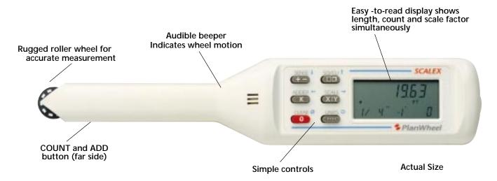
Measure plans the fast, accurate way with the Scalex Plan Wheel™. Here's the perfect tool for taking scaled measurements from blueprints, maps, and plans. Just select the built-in scale factor to match the plan and roll the Plan Wheel. The measurement is displayed instantly.
