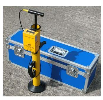
Introduction: - The 4.5 Kg CIST/883 Clegg Impact Soil Tester manufactured by SDi provides an easy and straightforward means for measuring and controlling soil strength and consolidation levels during trench reinstatement. The 883 readout is clamped to the guide tube and the displayed reading is viewed from the top during use. Single button operation design provided for easy use.
