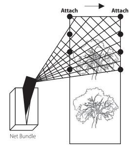
**2:** To achieve the FULL width, the net must be pulled ACROSS to the required width BEFORE it is attached along the side.
