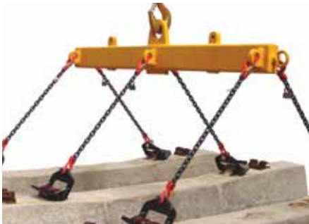
Image shows dropper chains terminating in Fastclip hooks
